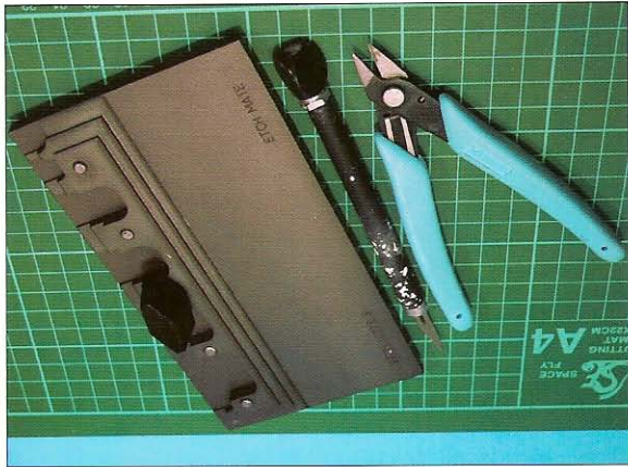
Here are the tools I use for photoetch work: a Xuron photoetch shear; a hobby blade; a cutting mat; and the Mission Models Etch Mate, for bending pieces of photoetch. (JA)
