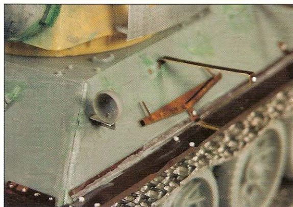
The headlight mounting bracket was made out of metal; the interior of the headlight was thinned out with a drill too. (MJ)
