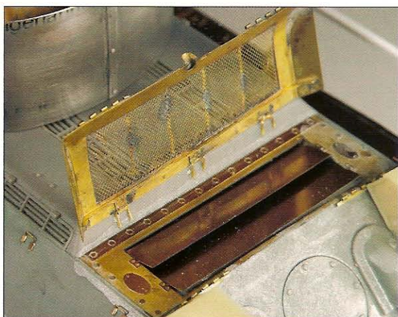
The interior cooling hatches are from the PART photoetch set, while the external metal grille is from Aber. (MJ)
