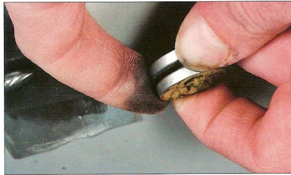
Graphite from a pencil was then rubbed onto the metallic paint using my finger. (AW)
