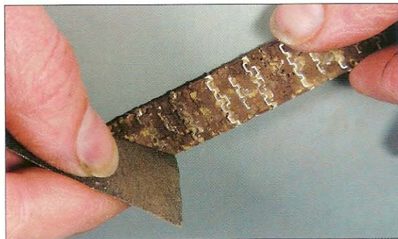
Having weathered the tracks, the outer parts were polished using sandpaper. (AW)
