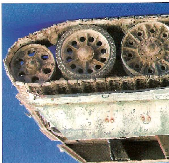
The drive wheel needed a bit of reworking so I carefully ground away the bolted roller details found on the outer surface of each wheel half. Once that tedious task was accomplished I sledged a bit of Mr. Surfacer 500 on the wheel to even things up a bit. (MK)
