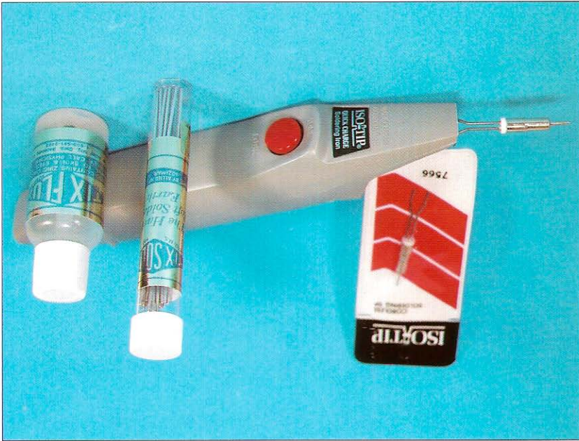
The items I use to solder photoetch: the cordless Iso Tip soldering iron with micro tip, Tix Flux, and Tix Solder. (A)
